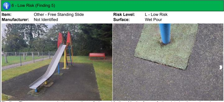
**Finding:** There are gaps opening between the surfacing and **Action:** Monitor for any further deterioration and repair as the edging surround or between the joints in the surfacing required
