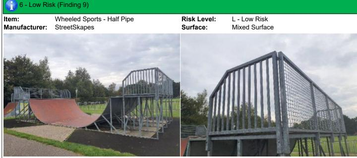
**Finding:** The height of the barrier is less than 1200mm and **Action:** Monitor - No remedial work recommended fails the requirements of BS EN 14974
