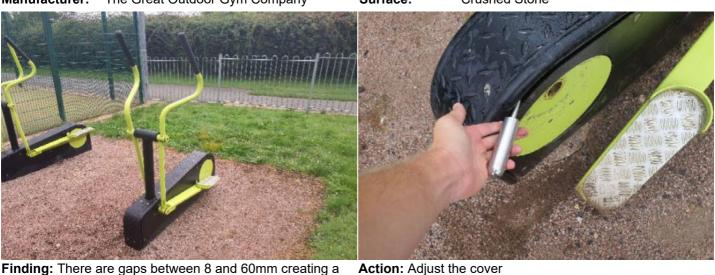
Finding: There are gaps between 8 and 60mm creating a potential crush/shear point in contravention of the requirements of BS EN 16630
