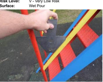
Finding: The item fails to meet the requirements of BS EN Action: Monitor - No remedial work recommended 1176 Part 1 4.2.7.2 for head and neck entrapment in the frame
