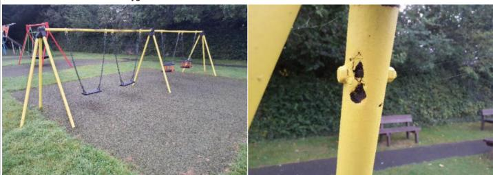
**Finding:** Parts of the steel on this item have corroded excessively and the metal has perforated in places
