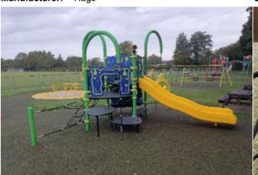
**Finding:** The item has been installed marginally too high which has resulted in the platform height being in excess of 600mm (610 mm) and technically, the height of the barriers are now insufficient to meet the requirements of BS EN 1176 Part 1. This is however a very low risk technicality and no remedial action is recommended as it has not affected the risk assessment of the item
